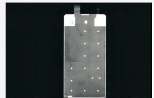
Film hole inspection on mobile cover
