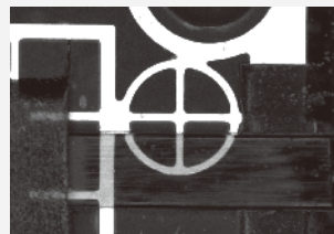
Mark locating for cutting
