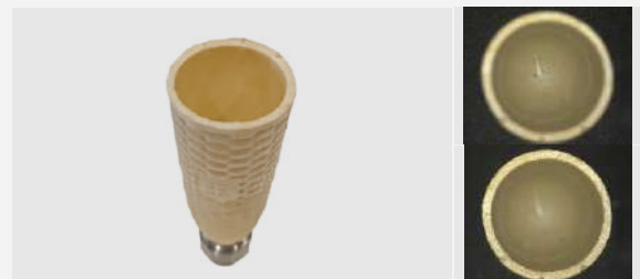
Ice cream cone exterior inspection-liquid lens testing
